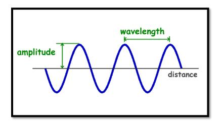
Amplitude is generally calculated by looking on a graph of a wave and measuring the height of the wave from the resting position.
