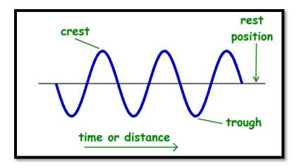
In this picture you can see that the highest point on the graph of the wave is called the crest and the lowest point is called the trough. The line through the center of the wave is the resting position of the medium if there was no wave passing through. We can determine a number of wave properties from the graph.
